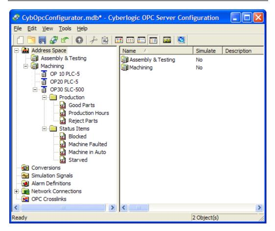
The "branches" of the tree are device folders, devices and folders. These establish how the data items are organized. The data items themselves are the "leaves" of the tree. You will begin construction of the tree at the address space root folder, which may contain device folders and devices.
