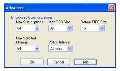
The default settings will typically provide for optimum operation of the driver. However, some situations may require these parameters to be changed. Refer to the Communication Using the DHX Driver section for more information.
