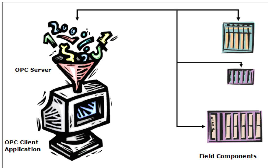
OPC servers obtain data from field components and present it, in a standard way, to OPC client applications. The basic functionality of the OPC server is the same for all types of field components and networks, but some of the communication and data-handling will vary from one family to another. The driver agent is a plug-in software module that accommodates these specific differences.
