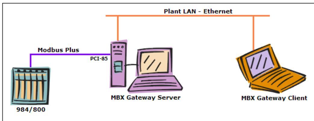
In this setup, the tower system uses the MBX Driver and a PCI-85 card to communicate over Modbus Plus to the 984 controller. The tower is also running the MBX Gateway Server, making it the server system.
